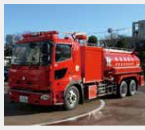
10-ton water tank truck
